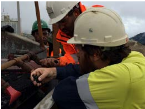
Evaluation of activated carbon at fine carbon removal.
