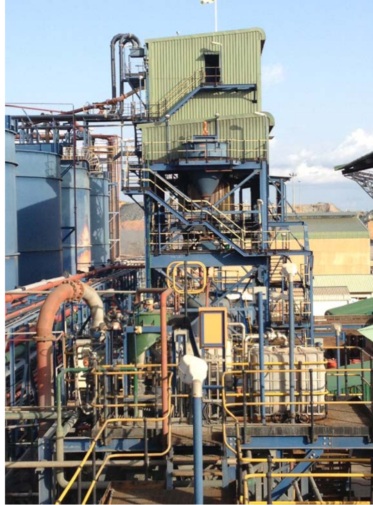
Leach tanks and elution column. Tongon Mine Cote d'Ivoire.
